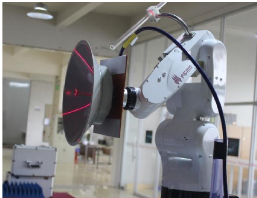
Fig. 4. Robotic Controlled Laser Toolkit for Coordinate Calibration
