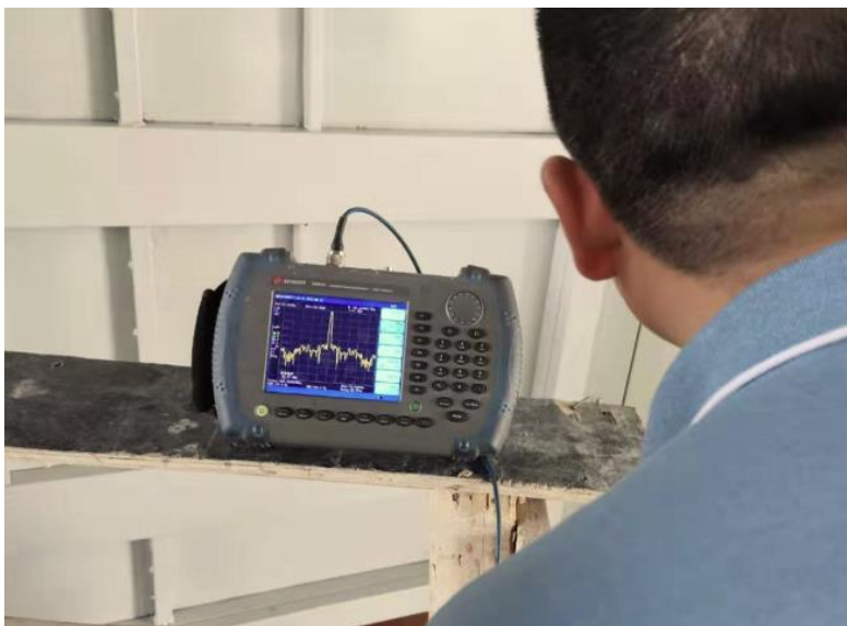
Fig. 3. F&MM Measurement for Shielding Quality of Anechoic Chamber
