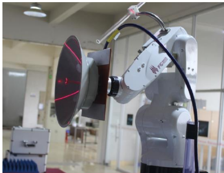
Fig. 4. Robotic Controlled Laser Toolkit for Coordinate Calibration
